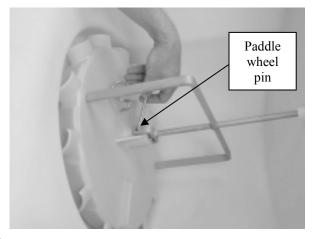
3 ...Then remove the paddle wheel pin by firmly rotating the pin and pulling upward.
